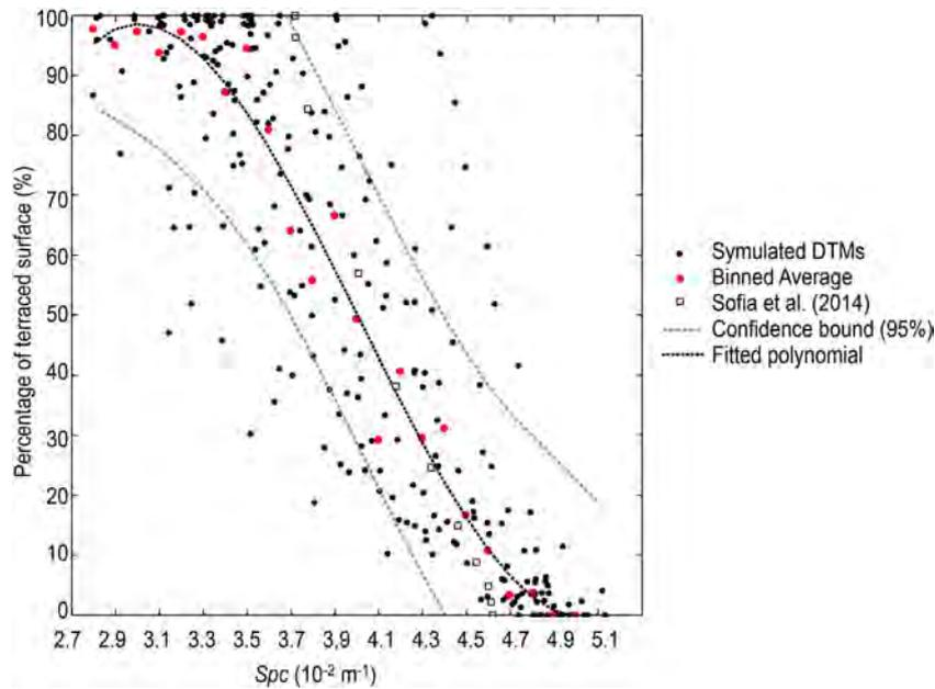
**Fig. 6.** Spc for the simulated DTMs, the binned average values and the derived curve fitting, as compared to the Spc for the Mediterranean dataset (Sofia et al., 2014). The 95% confidence interval is also shown.
