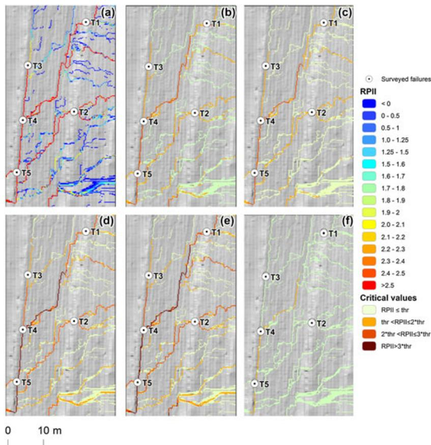
Figure 8. RPII for the TLS surveyed area (a) and extraction of critical values (b–f). The considered thresholds are the  $\sigma_{RPII}$  (b),  $IQR_{RPII}$  (c),  $MAD_{RPII}$  (d),  $Q-Q$  plot<sub>RPII</sub> (e) and outliers (f). This figure is available in colour online at [wileyonlinelibrary.com/journal/ldr](http://wileyonlinelibrary.com/journal/ldr)
