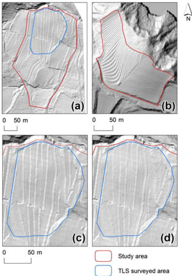
Figure 3. Available ALS DTMs at 1-m resolution for the Lamole (a) and the Pesaro (b) study areas, and comparison between the ALS 1-m DTM (c) and the TLS 0.2-m DTM (d) for the Lamole study area. This figure is available in colour online at [wileyonlinelibrary.com/journal/ldr](http://wileyonlinelibrary.com/journal/ldr)
