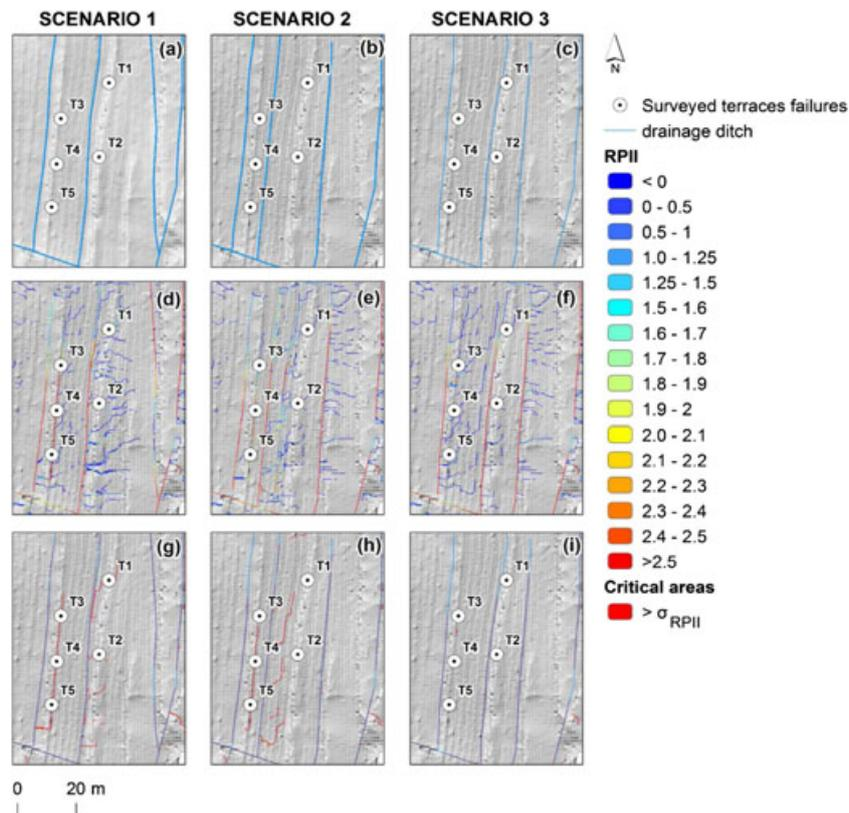
Figure 10. Lamole case study. Simulations of four different drainage ditch systems (a–c) and derived RPII maps (d and e). Figures from (f) to (i) show the critical areas, identified using  $\sigma_{RPII}$  as threshold. This figure is available in colour online at [wileyonlinelibrary.com/journal/ldr](http://wileyonlinelibrary.com/journal/ldr)
