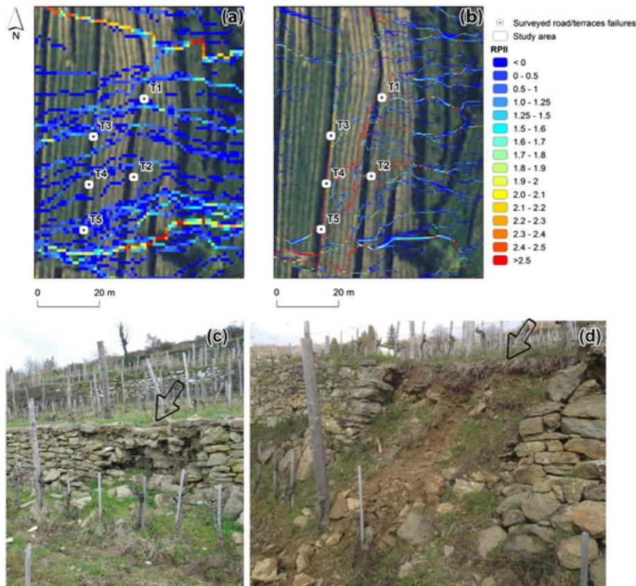
Figure 6. Lamole case study. RPII maps derived from the 1-m ALS DTM (a) and from the 0.2-m TLS (b), highlighting the flow modifications induced by the terraced structures, and the related terraces failures (T1 in (c) and T5 in (d)). This figure is available in colour online at [wileyonlinelibrary.com/journal/ldr](http://wileyonlinelibrary.com/journal/ldr)
