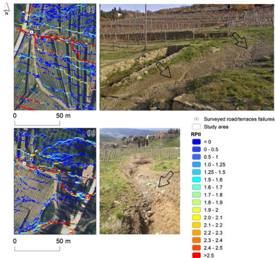
Figure 5. Lamole case study. RPII maps derived from the 1-m ALS DTM, highlighting the flow modifications induced by the road, resulting in road erosion. This figure is available in colour online at [wileyonlinelibrary.com/journal/ldr](http://wileyonlinelibrary.com/journal/ldr)
