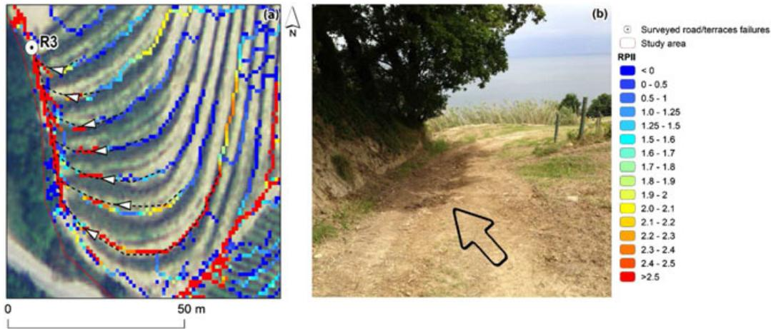
Figure 7. Pesaro case study. RPII maps derived from the 1-m ALS DTM (a) highlighting the flow modifications induced by the terraces, causing water accumulation that erodes the road (b). This figure is available in colour online at [wileyonlinelibrary.com/journal/ldr](http://wileyonlinelibrary.com/journal/ldr)
