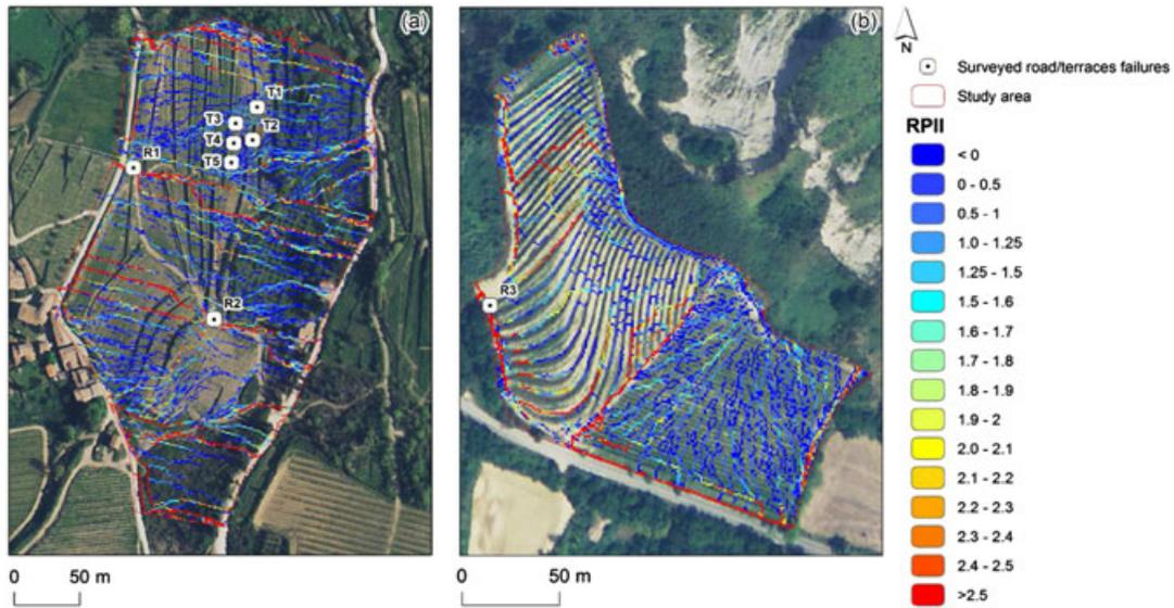
Figure 4. RPII maps derived from the 1-m ALS DTM for the Lamole case study (a) and the Pesaro case study (b), with surveyed terraces instabilities (T1 to T5) and eroded roads (R1 to R3). This figure is available in colour online at [wileyonlinelibrary.com/journal/ldr](http://wileyonlinelibrary.com/journal/ldr)
